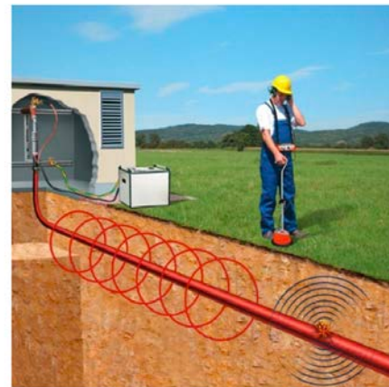
Figure 12. Pinpointing faulted cable.
